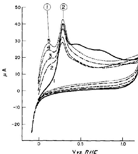
Fig. 2.  $i$ - $E$  diagram of nickel in 0.1 M KOH electrolyte; sweeprate  $10 \text{ mV} \cdot \text{s}^{-1}$ . Before the 1st sweep Ni was polished and cathodically polarised; between each successive recorded sweep, a potential sweep 0–300 mV was applied.
