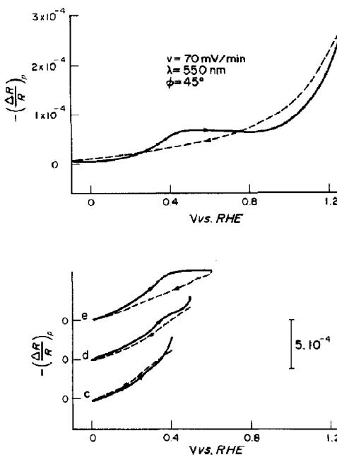
Fig. 8.  $(\Delta R/R)_0$  as a function of increasing and decreasing potential for increasing anodic return potentials.
