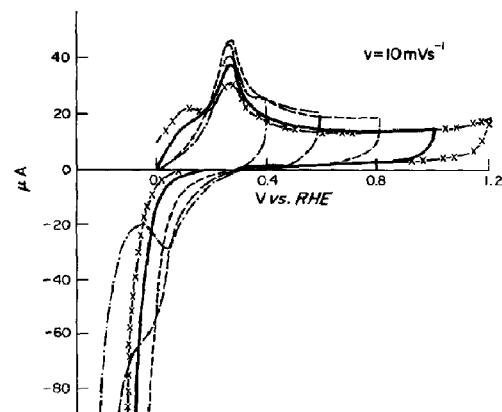
Fig. 4. Effect of increasing anodic return potential; sweeprate  $10 \text{ mV} \cdot \text{s}^{-1}$ . —  $E_{\text{return}} = 400 \text{ mV}$ ; - - -  $E_{\text{return}} = 600 \text{ mV}$ ; - · -  $E_{\text{return}} = 800 \text{ mV}$ ; —  $E_{\text{return}} = 1000 \text{ mV}$ ; -  $\times$  -  $E_{\text{return}} = 1200 \text{ mV}$ .
