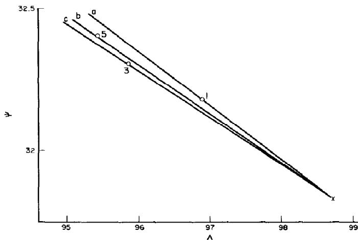
Fig. 9. Calculated  $\Delta, \psi$  plots for  $\text{Ni}(\text{OH})_2$  film with refractive indices: curve a :  $n - ik = 1.45 - 0.01i$ ; curve b :  $n - ik = 1.50 - 0.02i$ ; curve c :  $n - ik = 1.55 - 0.03i$ . The points in the figure are the experimental data of Fig. 7.
