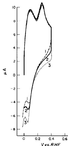
Fig. 6. Effect of oxidation time at  $E_{\text{return}} = 400 \text{ mV}$  upon the reduction cycle (sweeprate  $2 \text{ mV} \cdot \text{s}^{-1}$ ).
