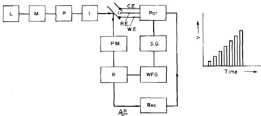
Fig. 1. Schematic diagram of electrochemical spectro-reflectance apparatus. L: Tungsten lamp; M.: monochromator; P.: polariser; l.: lenses; PM.: photomultiplier; Pot: potentiostat; S.G.: scan generator; Rec.: recorder; W.F.G.: wavefunction generator; R: measurement of  $\Delta R/R$ ; C.E.: counter electrode; R.E.: reference electrode; W.E.: working electrode (Ni).
