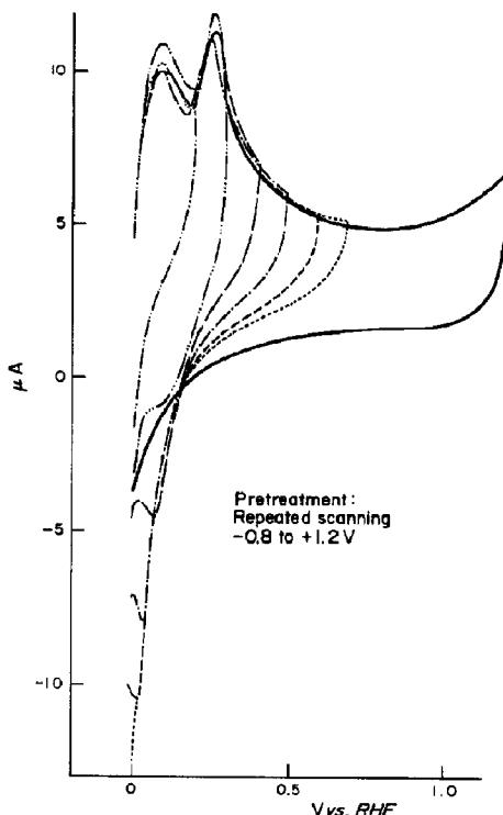
Fig. 5. Effect of increasing anodic return potential on a "stabilized" Ni electrode (sweeprate  $2 \text{ mV} \cdot \text{s}^{-1}$ ). —···  $E_{\text{return}} = 160 \text{ mV}$ ; —··—  $E_{\text{return}} = 300 \text{ mV}$ ; ———  $E_{\text{return}} = 400 \text{ mV}$ ; ———  $E_{\text{return}} = 500 \text{ mV}$ ; ———  $E_{\text{return}} = 600 \text{ mV}$ ; ······  $E_{\text{return}} = 700 \text{ mV}$ ; ———  $E_{\text{return}} = 1200 \text{ mV}$ .
