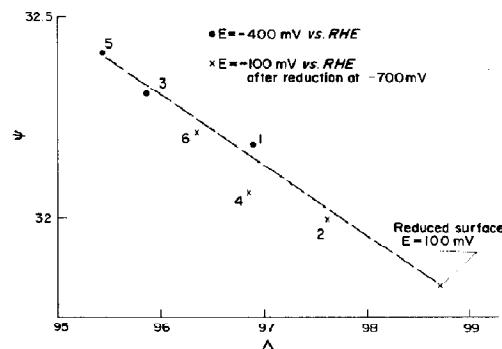
Fig. 7. Change of the ellipsometric parameters with repeated oxidation (at 400 mV) and reduction at -700 mV. After reduction the measurement was carried out at -100 mV. The numbers denote the subsequent processes.
