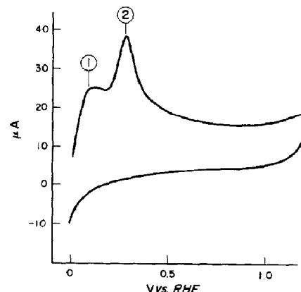
Fig. 3. Voltammogram of Ni in 0.1 M KOH after 11 potential sweeps from -800 to 1200 mV; sweeprate  $10 \text{ mV} \cdot \text{s}^{-1}$ .
